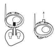
To detach the BTCity, simply press the fixing clip and push the unit upwards.
