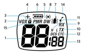
Your **Midland G9 PRO** keeps you constantly updated about its operational status through a Liquid Crystal Display (LCD). The symbols and their corresponding parameters that may appear, according to the operational status of the device, are described as follows:
