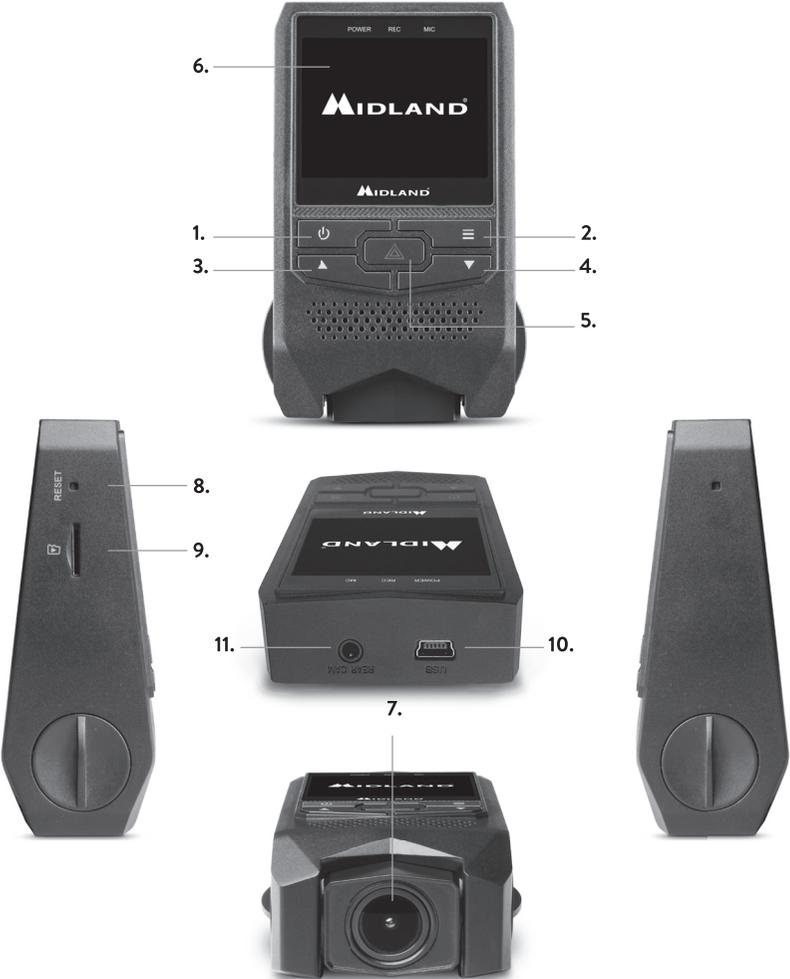
1. **⏻ ON/OFF:** Press shortly to turn on the camera; keep pressed to turn it off.
