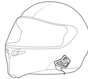
Place the **BT Mini** unit on the left side of your helmet using the adhesive mount.
