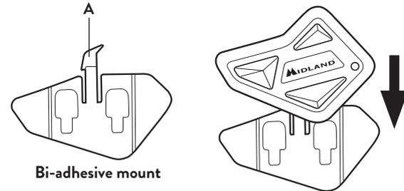
The **BT Mini** can be easily fitted onto the helmet by sliding it downwards into the slot of the adhesive Mount.
