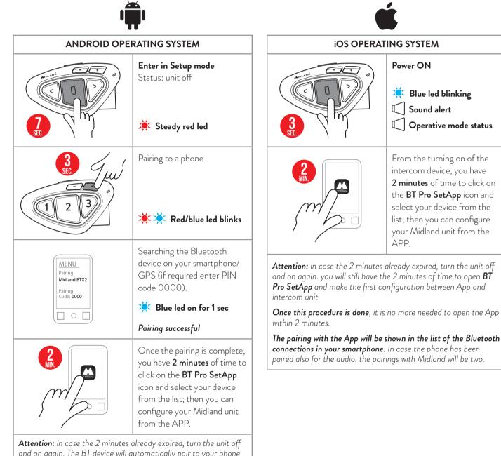
and on again. The BT device will automatically pair to your phone and you will still have the 2 minutes of time to open **BT Pro SetApp** and make the first configuration between App and intercom unit.
