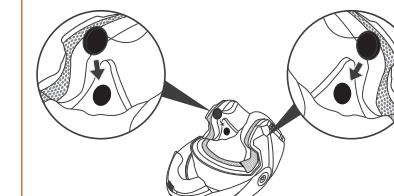
The **BTX1 PRO S** can be easily fitted onto the helmet by sliding it downwards into the slot of the adhesive Mount.
