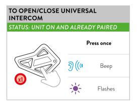
**Note:** to open/close the audio with a different brand device, use the voice call command (for some models, it is required to send the voice call twice).
