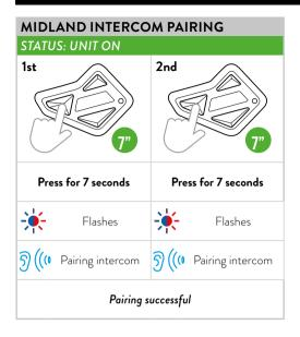
**Note:** By following the same procedure, it is possible to pair two further devices to the **Up or Down** buttons.
