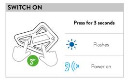
**Attention:** upon turning on or off, pressing the two button longer than the indicated time could reset the pairings.
