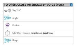
**Note:** Voice activation is only possible with an intercom paired with the **down button** (Vox must be active).
